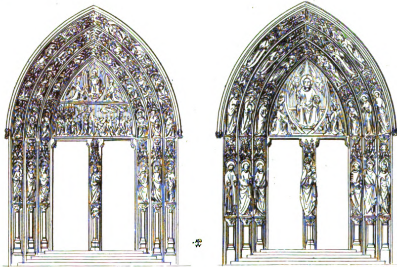
Illustration of the different effects of scale produced by large or small statues in the same space.
